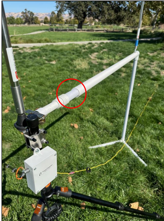
Each band requires different element lengths (director is always 6% shorter ) and element spacing . The horizontal PVC tube telescopes like a trombone to accommodate band spacing.
