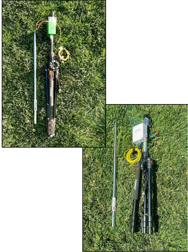
The LDG™ 4:1 unun or the TennTennas™ 49:1 with RF choke are already mounted to the tripod for fast and easy deployment.
