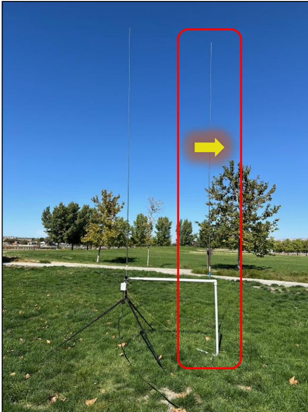
Dominator 2-Element Vertical Beam for 10M pointed east at US-3473 in California. Parasitic director creates up to +4 dB gain across four bands: 17M-10M.
