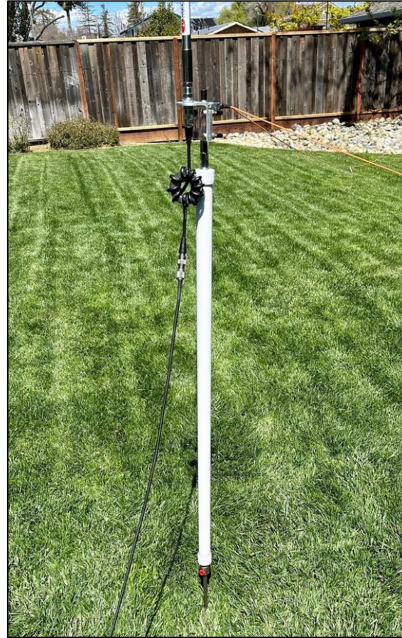
PERformer shown with a 40" furniture-grade PVC tube on a Chameleon™ ground spike.
