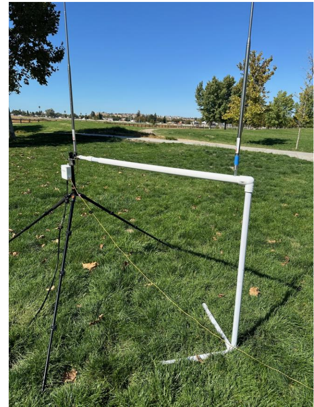
Horizontal PVC section rests on top of the tripod mirror mount which can be manually rotated to any direction. The counterpoise wire runs under director .
