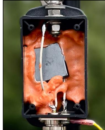
Bullet-4U-100 Dual 1/4" Port Ferrite Bead Mix 43 1.125" Height x 1.125" Width x 0.5" Depth
